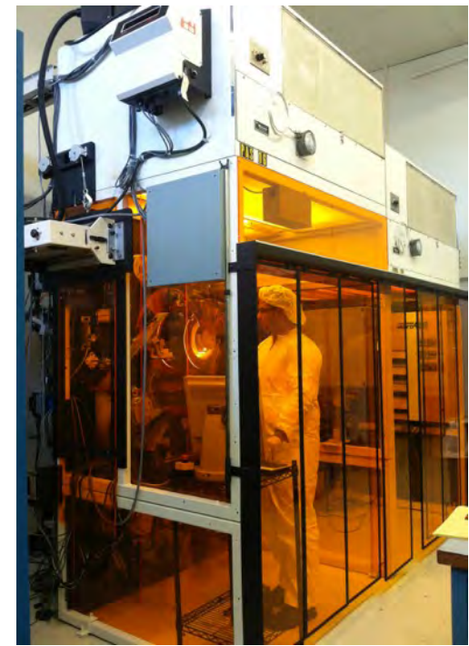
GEN-3 R2R nanoimprinter
